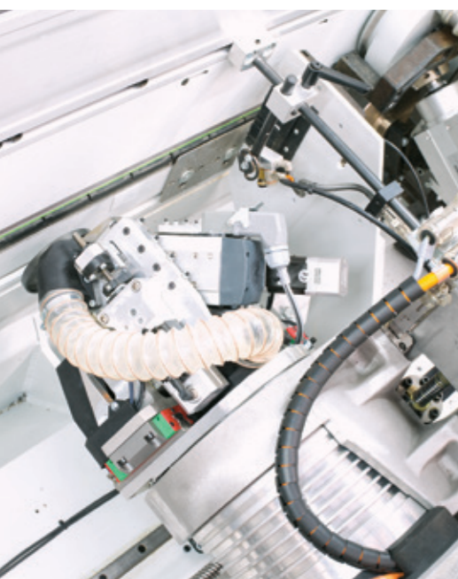
The AR70 is a single-motor corner-rounding unit that gives you the advantage of being able to do two-radius corner-rounding.
